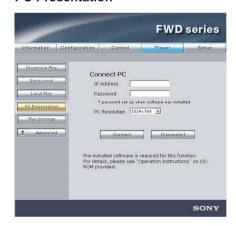
This screen lets you start and stop the PC Presentation function of the BKM-FW50. By showing the contents of the computer desktop on the display, the PC Presentation function allows using the display as an external monitor for the computer.
